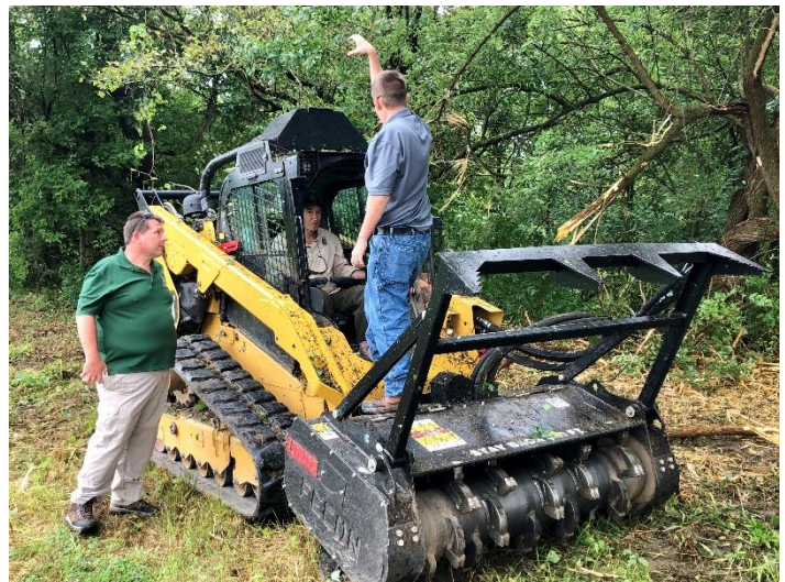
Members of the HCP&R maintenance crew prepare to use a FECON forestry mulcher to clear invasive plants and trees at W.S. Gibbs Memorial Park.
