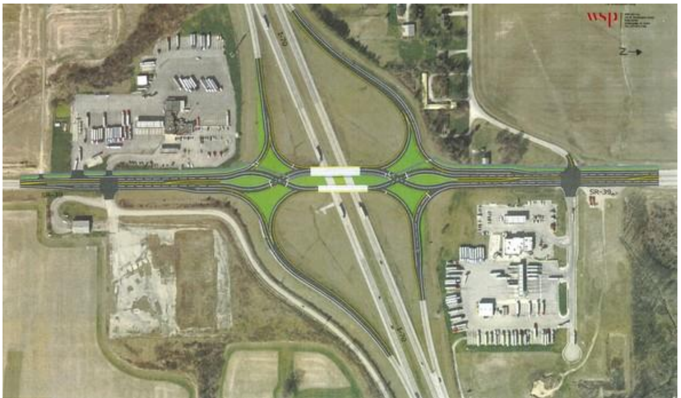
Conceptual drawing of DDI at I-70 and SR 39. Source: Indiana Dept. of Transportation.
